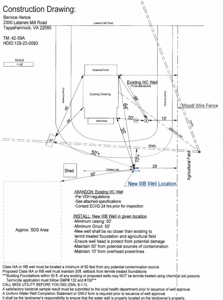
See attached abandonment specifics. If abandonment is required, documentation of such is required on a Uniform Water well Completion Statement or GW-2.
